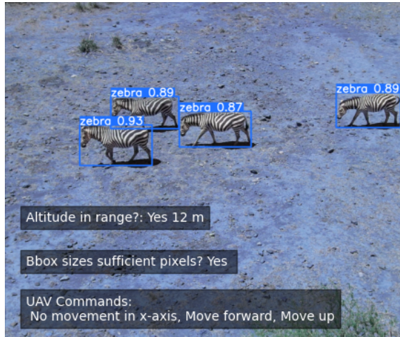
Figure 3: Example Autonomous Navigation Model Output
